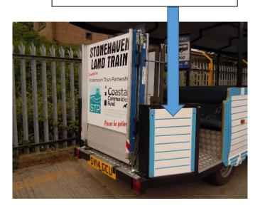
2. This shows one of the side panels which has a light in the middle. There is space for two adverts on each of these they measure 50cm wide by 25 cm deep for the top one and are a little deeper at the bottom 25-30cm deep with a slight curve at the bottom.
